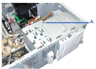
Figure 4 - 21 : HDD Bracket Screw
